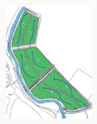
The reed beds, planted in open water, have been arranged in a series of cells, each surrounded by raised earth 'berms'. Water is brought in via two equal flow paths, which each travel through three reed cells. A portion of excess nutrients are removed from the water through a combination of sedimentation, plant growth and denitrification processes.
